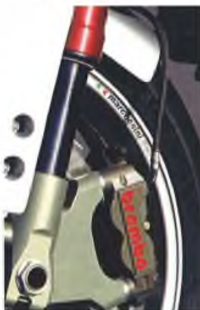
v Fully adjustable Marzocchi USD fork fits twin Braking/Wave rotors and radial-mount 4-pot Brembos. Note the ultra rigid calliper mount and Marchesini scripting on magnesium wheel. The ultimate track day weapon?
