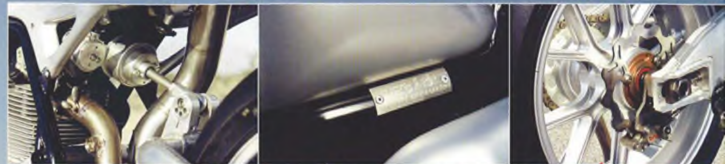
^ (left) "Old school" cantilever joins the Millona's trick, tig-welded aluminum swingarm to a Double-System pneumatic monoshock. Simple and effective, an eccentric on the shock mount allows adjustments for ride height and shock angle. For those desiring a more traditional unit, a choice of dampeners is offered. (middle) Produced in limited numbers, Poggipolini/NCR will manufacture twelve Ducati 1000DS powered Millona in 2005, with only four coming stateside. Cost is 30K€. (right) A major factor in keeping the Millona light and strong are these forged magnesium wheels, Braking and Brembo components highlight arthful craftsmanship.
