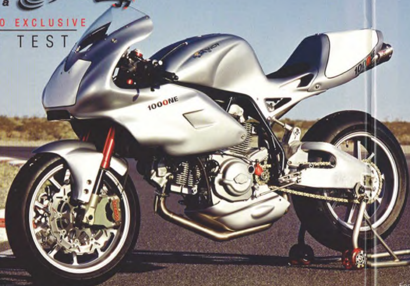
^ (left) "Old school" cantilever joins the Millona's trick, tig-welded aluminum swingarm to a Double-System pneumatic monoshock. Simple and effective, an eccentric on the shock mount allows adjustments for ride height and shock angle. For those desiring a more traditional unit, a choice of dampeners is offered. (middle) Produced in limited numbers, Poggipolini/NCR will manufacture twelve Ducati 1000DS powered Millona in 2005, with only four coming stateside. Cost is 30K€. (right) A major factor in keeping the Millona light and strong are these forged magnesium wheels, Braking and Brembo components highlight arthful craftsmanship.
