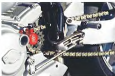
^ A key to the Millona's handling prowess is this strengthened swingarm pivot that uses both the frame tab and engine case; long a standard feature on Ducati's Superbike models.
