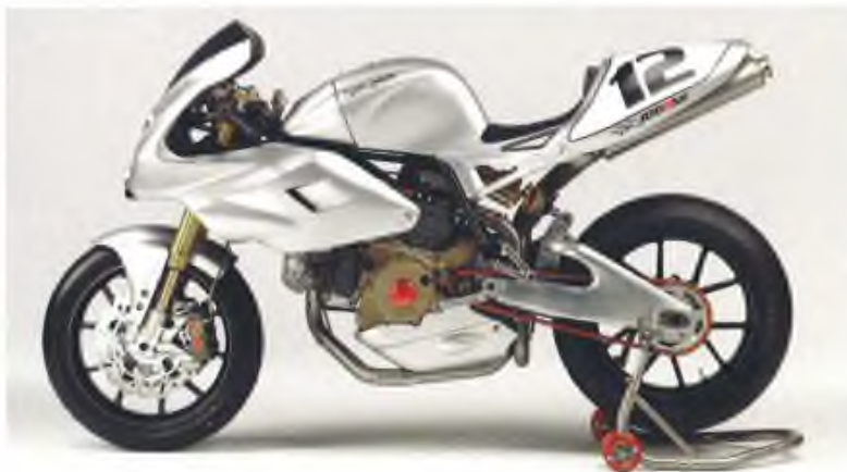
^ With a rich history in developing high performance Ducati-powered specials and historic racing motorcycles, NCR introduces the Millona; a machine for the new generation of Ducatisti. Our test unit uses a mostly stock, air-cooled, 2v 1000DS Supersport engine, a perfect test bed for NCR's line of high performance accessories aimed at ST and Multistrada owners. Lightness and attention to detail make it work.
