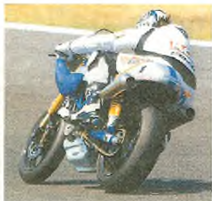
Zard exhaust weighs just 4kg – a third of standard system
